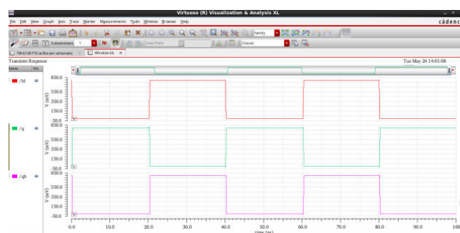
Fig.7. Simulation result of transient analysis for Single ended 9T SRAM Cell.
