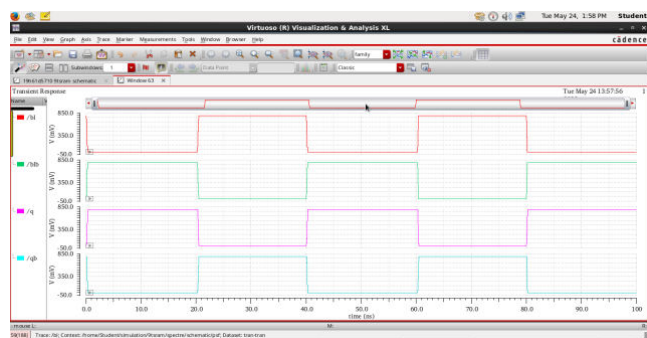
Fig.3. Simulation result of transient analysis for 9T SRAM Cell.
